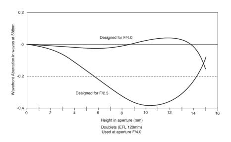
If a doublet designed for a high relative aperture is stopped down, then the image quality will improve. However the presence of the undercorrected primary aberrations, which it was necessary to introduce, will always make the performance inferior to that of a doublet which was designed for the target aperture. The effect is illustrated by the example of two Ealing doublets of focal length 120mm used at F/4.0, (see figure below.)
